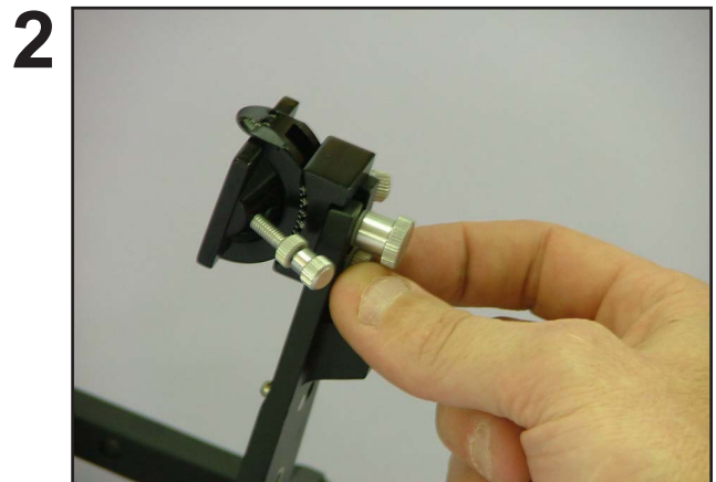
Place adjustable incisal table and lock in place with small thumb screw.
