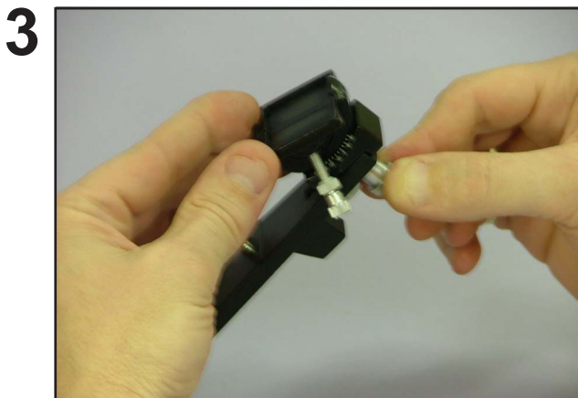
Adjust incisal guidance desired and lock in place with large thumb screw.
